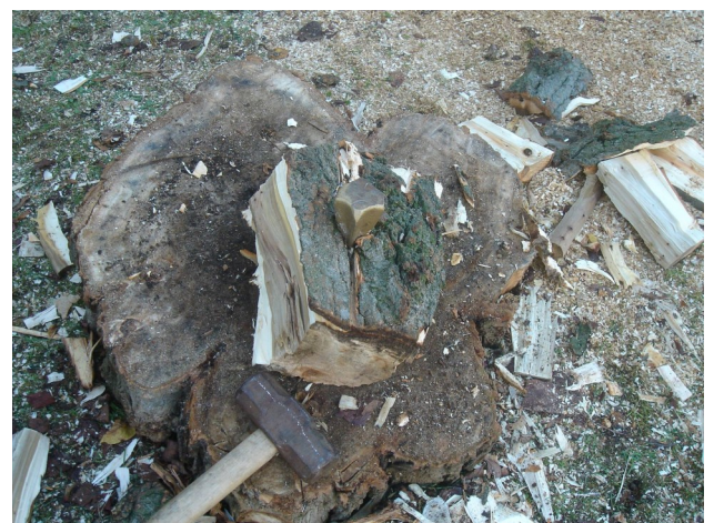
The splitter's called a grenade. Give me two for when the first one disappears inside the knotty log
